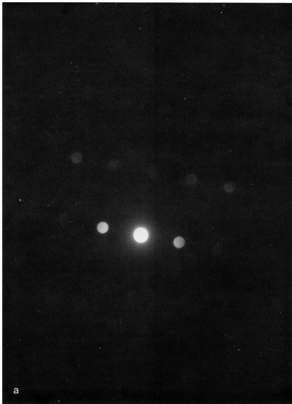
FIG. 5. (a) Electron microdiffraction pattern using a 5-nm electron probe from a PtSn (hcp) particle in CAT-B. (b) The solution for the observed pattern shown above. ( \Delta ) observed reflections, ( \circ ) calculated reflections, and (X) forbidden reflections, which appear due to double diffraction.
